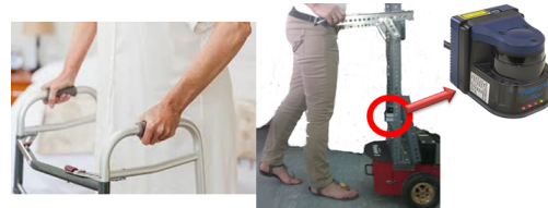
Fig. 1. Left: Typical passive assistive device for elderly. Right: A robotic platform based on Pioneer Robot equipped with a Hokuyo Laser Sensor aiming to record the gait cycle data of the user (below knee level).
